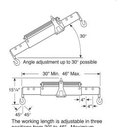
The working length is adjustable in three positions from 30" to 46". Maximium chain angle is 45°.
